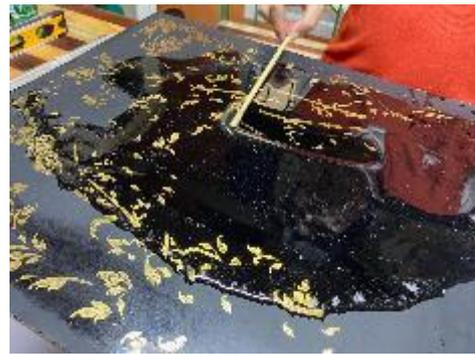
**Figure 2:** Coating with epoxy resin.
