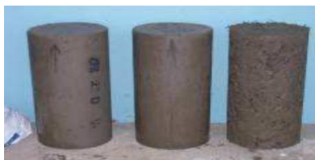
Figure 3. Concrete samples with different percentages of sugarcane bagasse fiber. Source: Hernandez, 2008.
