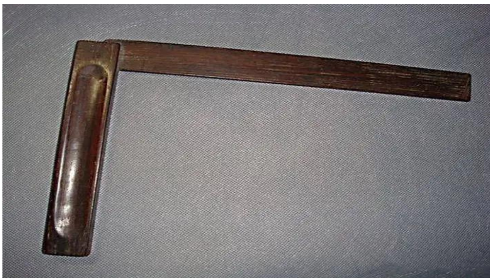
Figure 6. Tri-square(L-shaped drawing tool).
