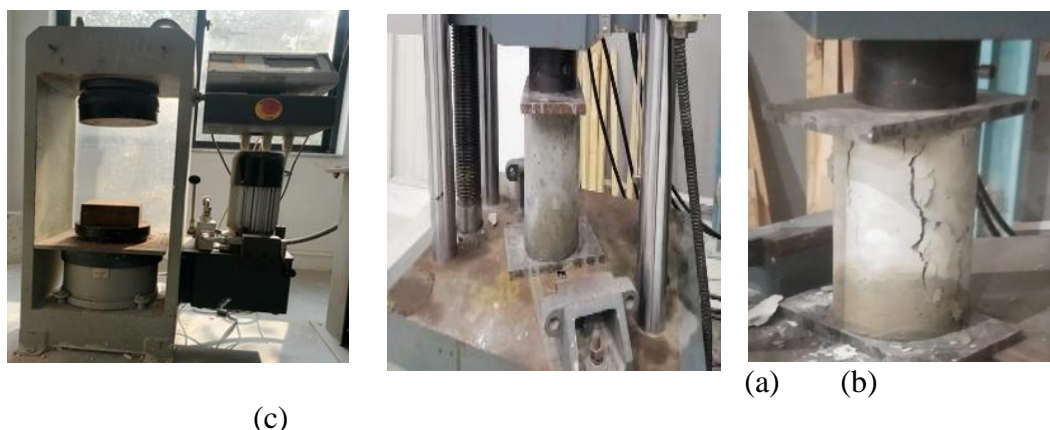
Fig. 6: Experimental setup (a) Compression Testing Machine (b) sample before testing & (c) sample after testing
