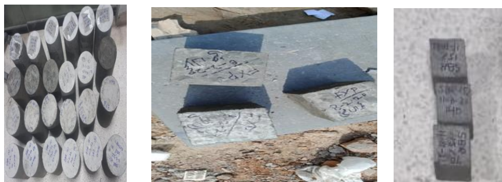
Fig. 4: After casting hardened concrete cylinders, cubes and mortar bars
