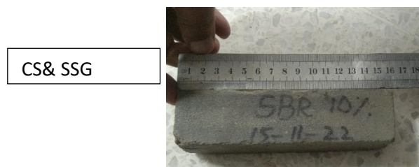
Fig. 8: Measurement of change in length of mortar bar
