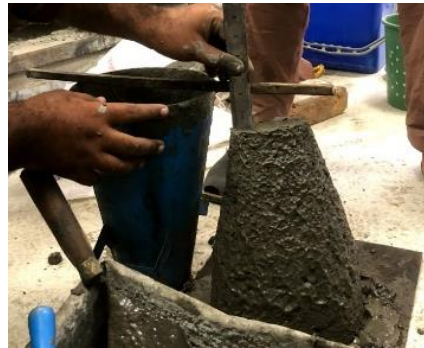
Fig. 5: Measurement of slump on fresh concrete
