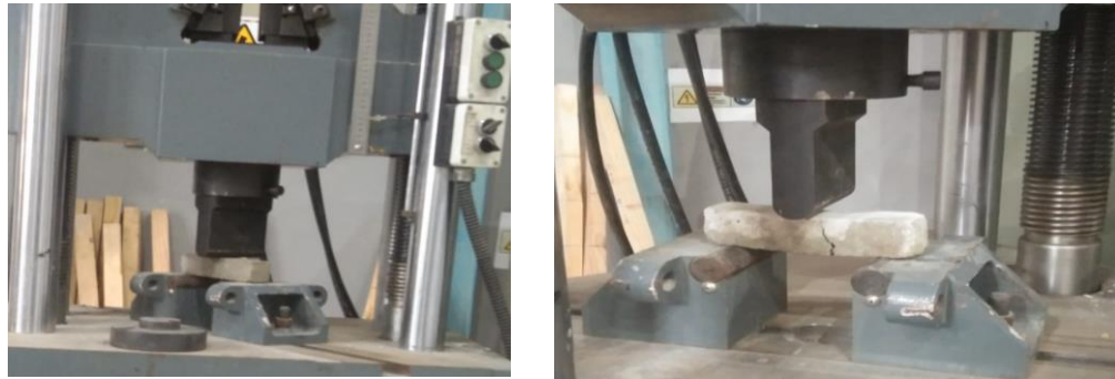
(a) (b) Fig. 7: Experimental setup: (a)Sample (mortar bar) before testing& (b) after testing
