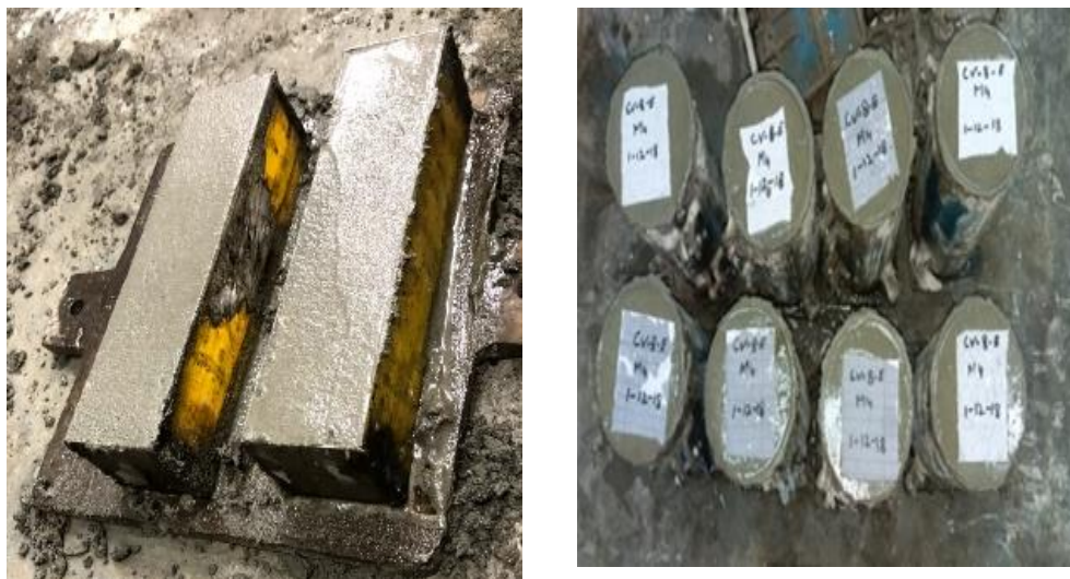
Fig.3: Casting of concrete cylinders, cubes and mortar bars
