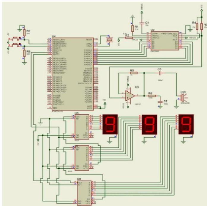
**Figure 2. Interfacing of seven segments**
