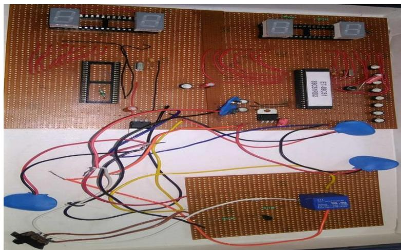
**Figure 5. Hardware of automatic token display system**
