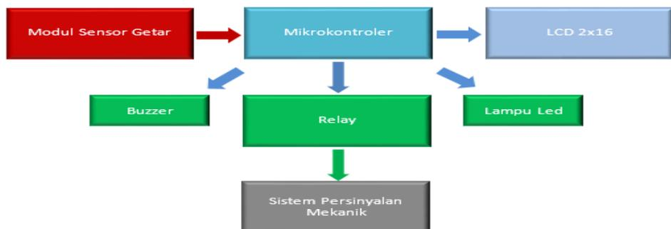
**Figure 5:** System Block Diagram
