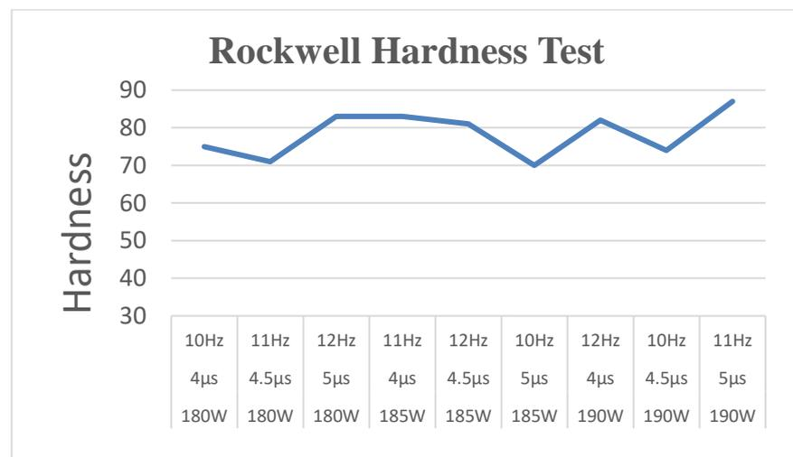
Fig. 1: Rockwell Hardness results
