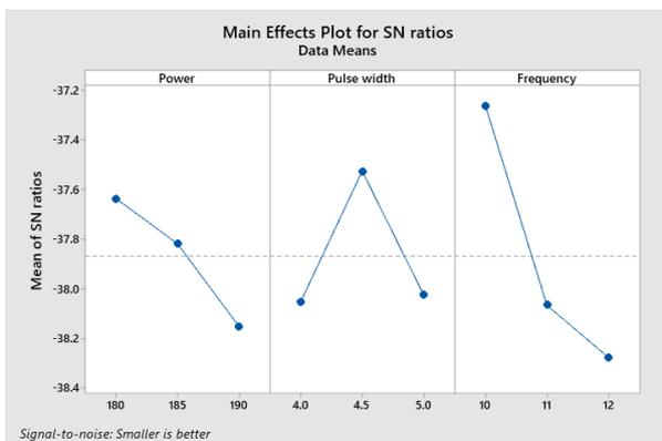
Fig. 2: Main effects plot for S/N ratios
