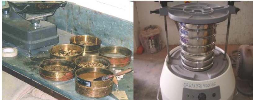
Figure. 7: B.S. sieve set and mechanical sieve shaker
