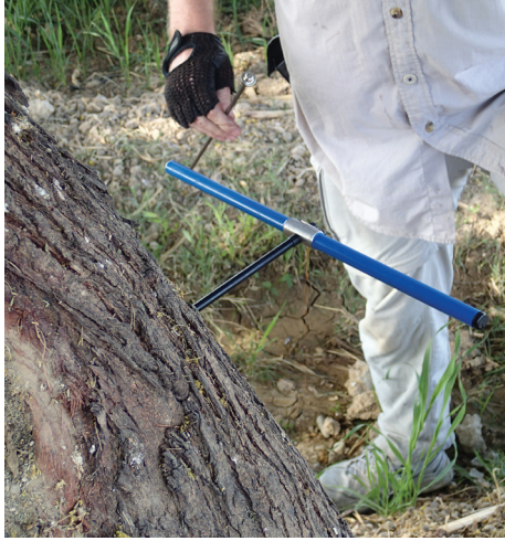
Figure 50b. Increment borer in use on Acacia sp. Photo by P.P. Creasman.
