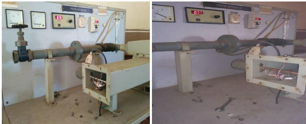
Fig1: Experimental setup of pin-fin apparatus
