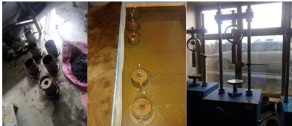
Figure 4.4: Sample procedures and tools in CBR test of this study
