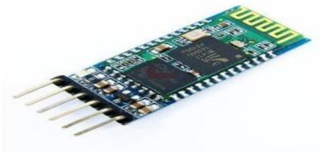
Picture 2.4. Bluetooth module HC-05 (Source: Robotic, 2020)
