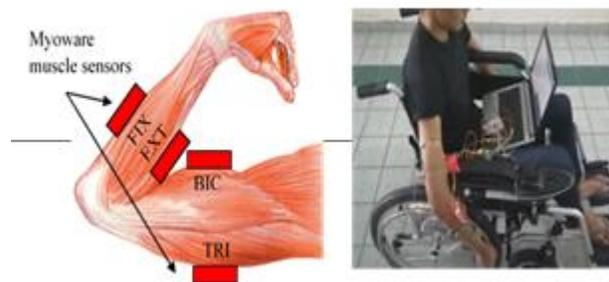
**Figure 6.** Placement of 4 Myoware muscle sensors on BIC, TRI, EXT and FIX muscles
