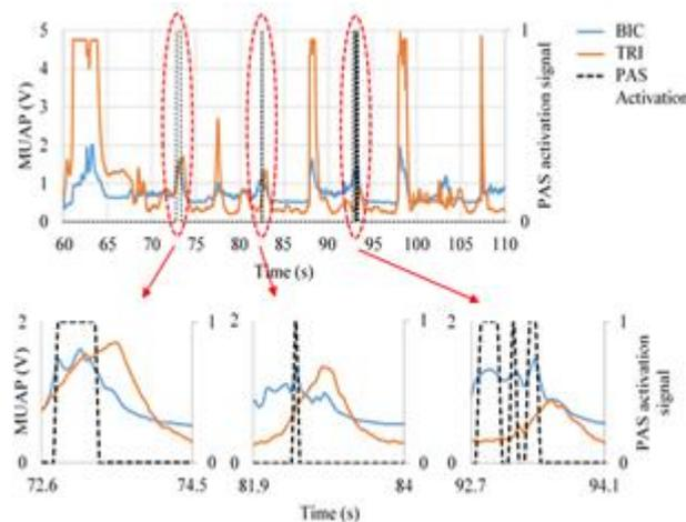
**Fig. 7.** PDF control method performance for subject 1 based on BIC & TRI MUAP signals
