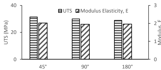
Fig. 11 A comparison UTS value and Modulus Elasticity at line pattern structure at a different angle
