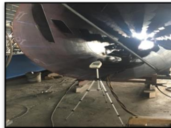
Figure 3 Set up for Sound Pressure level
