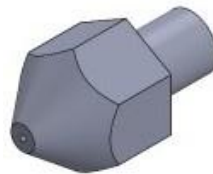
Fig. 2 The working design of 3D printer nozzle [7]
