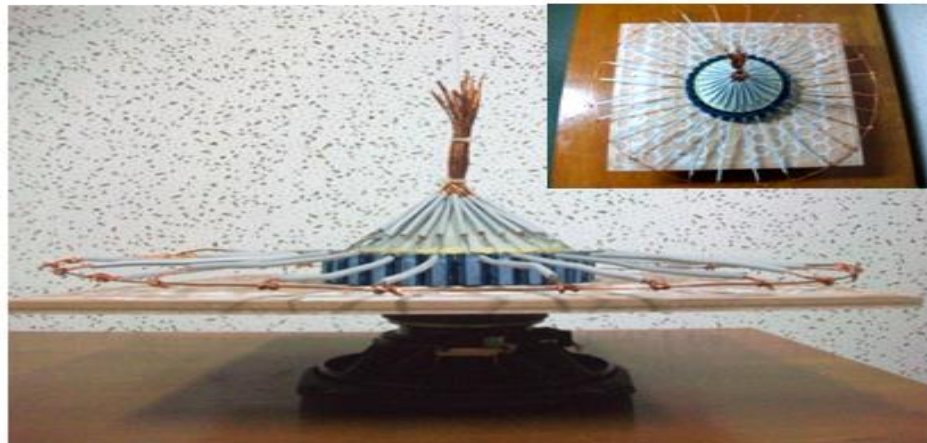
Figure 10 28 Electrolytic Capacitors Pooling Together to 54.7 Degrees (Magic Angle)
