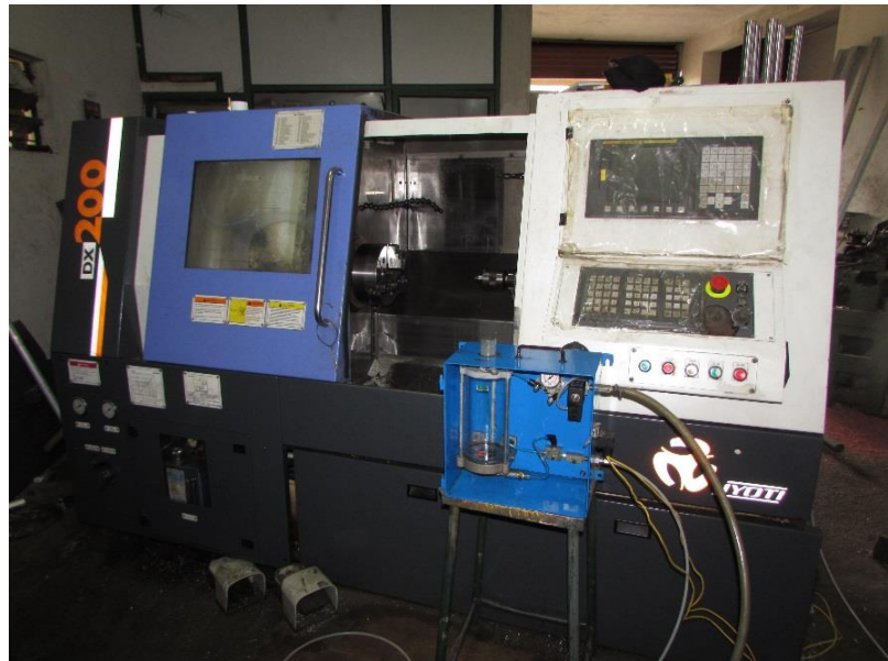
Figure 1. Machining setup with MQL system
