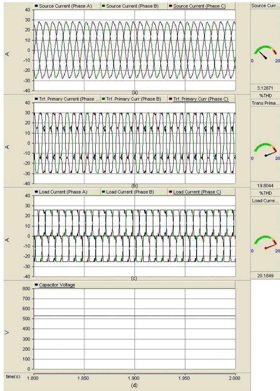
Fig.9.PSCAD/EMTDC results of the CT with APF.(a) Current at the load side. (b) Current in the PCC Point .(c) Current at the source side
