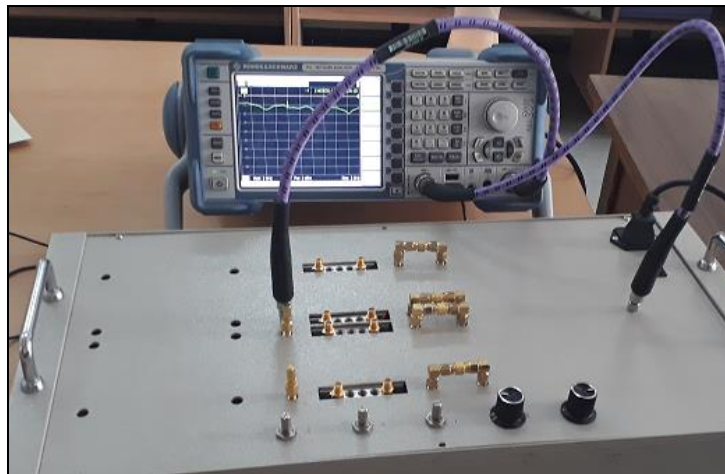
Fig.4: Experimental set up to measure S- parameters of phase shifter IC 2484 using VNA
