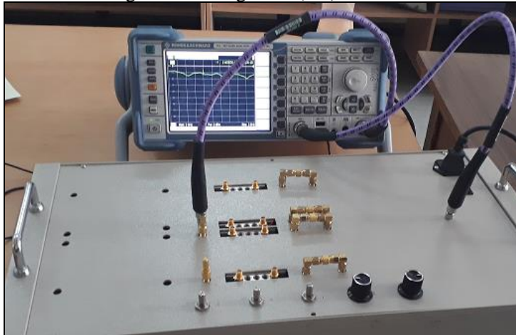
Fig.4: Experimental set up to measure S- parameters of phase shifter IC 2484 using VNA
