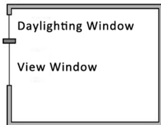
Figure 9: Daylighting Windows vs. View Window (Source: CHPS, 2002)
