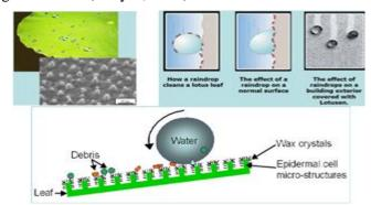
Water forms droplets on the tips of the epidermal protrusions of the Lotus leaf and collect dirt and pollutants as it rolls down the leaf. Same quality has been adopted in the Lotusan Paint
