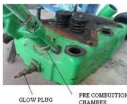
Fig.1. Modifications in Cylinder Head
