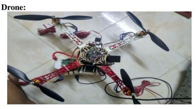
We have used a Generic Eachine H8 Mini RC Quadcopter controller in this drone to control all the movements of the drone. Drone primary controls are pitching, yawing and rolling.
