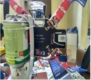
The spraying unit is used for spraying the pesticides on the weeds that are present on the crops. The weeds are identified using camera and with the help of image processing technique. The spraying is controlled a relay that is controlled by the raspberry pi 3 controller. Raspberry pi 3 is the most important part of this node. It is responsible for all the actions of the seeding and spraying unit. All the programs are stored in the Raspberry pi 3.
