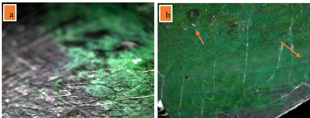
Figure 2 (a,b) : ( a ) : shown change in the color with detail from the higher left illustrating the darkened , ( b): shown bleaching spots on the surface and cracked
