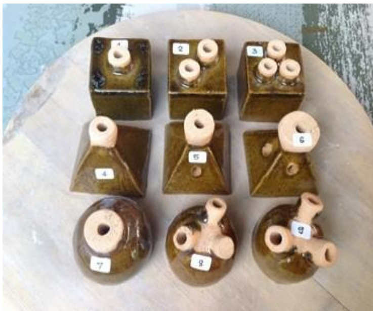
Figure 5 the clay body formulas gained from the experiments are casted into various shapes and forms with holes drilled to test about the essential oil evaporation rate.
